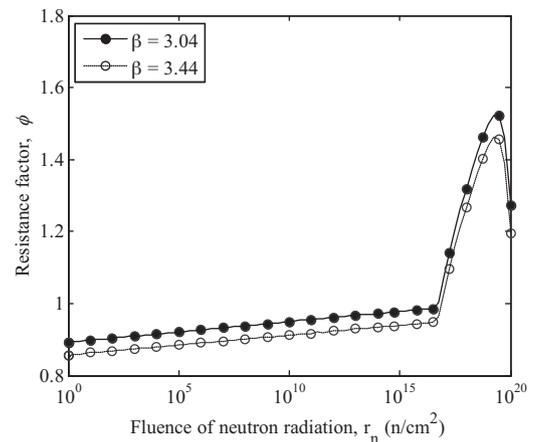
Fig. 5. Resistance factors for the target reliability indices,  $\beta = 3.04$  and 3.44 considering tension-controlled failure data.
