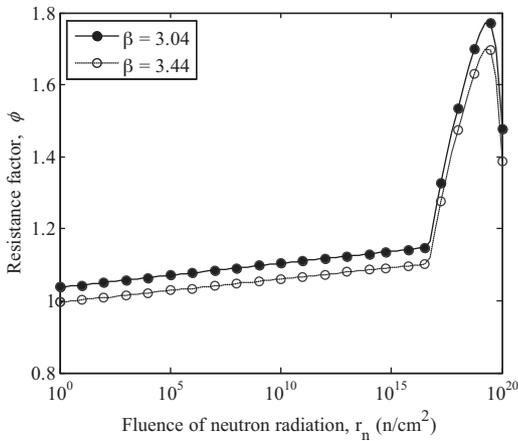
**Fig. 6.** Resistance factors for the target reliability indices,  $\beta = 3.04$  and  $3.44$  considering tension-controlled failure data and the upper limit (400 MPa) for the design yield strength of steel.
