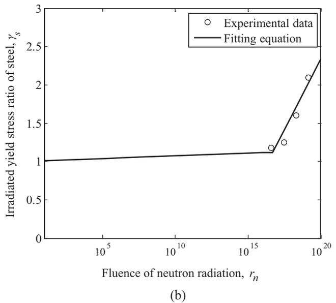
Fig. 2. (a) Uniaxial tension test results (Murty, 1984b) and (b) the yield strength ratio with respect to the fluence of neutron radiation.
