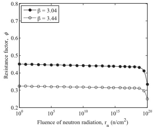
**Fig. 8.** Resistance factor for the target reliability indices,  $\beta = 3.04$  and  $3.44$  considering compression-controlled failure data.
