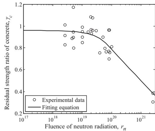
Fig. 1. Change of the compressive strength ratio of concrete with respect to the fluence of neutron radiation (Hilsdorf et al., 1978).
